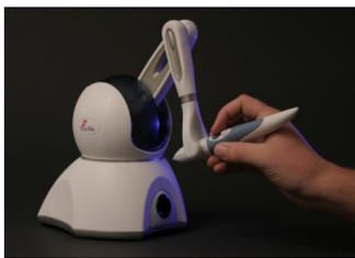
Figure 2: Phantom® Omni™ Device
