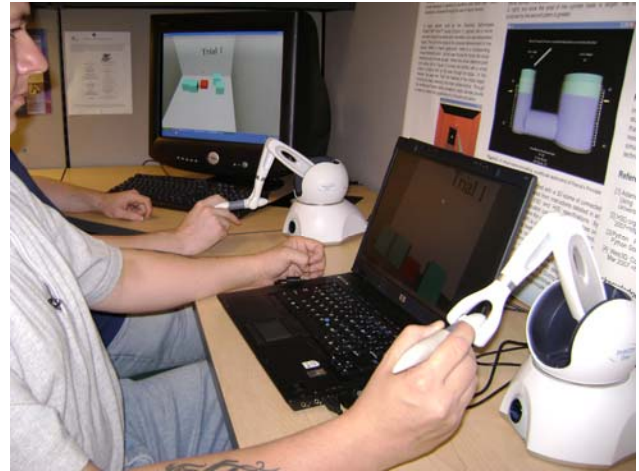
Figure 2. Two participants collaborate to stack a set of cubes. Each participant can manipulate one haptic pointer. In order to pick up the cubes they have to coordinate their moves.
