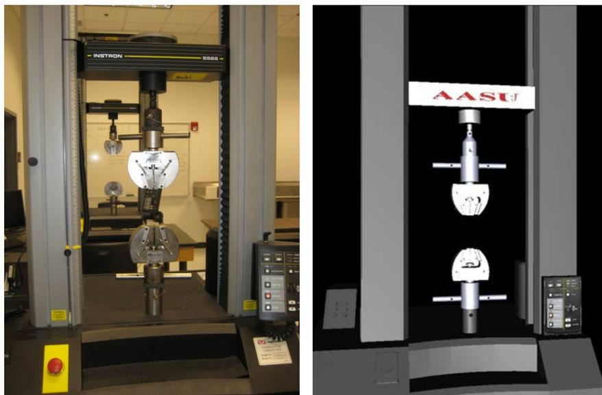
Figure 1: Instron™ 5566 real TTM (left) and simulator (right)
