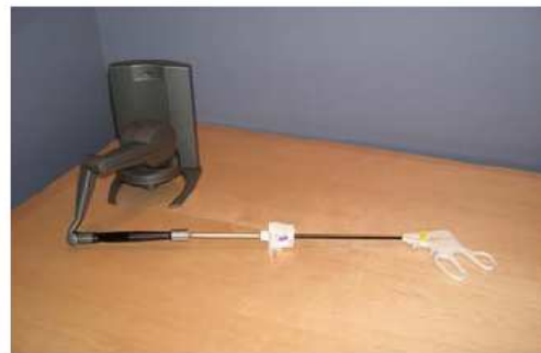
The PHANTOM Desktop haptic device with the Auto Suture® 5mm Endo Clinch® II device attached.
